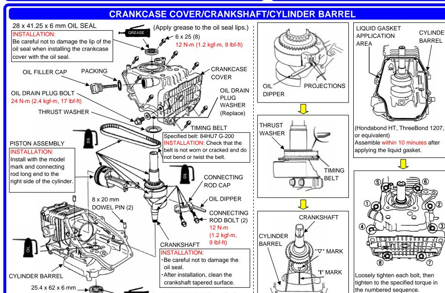
(Apply grease to the oil seal lips.)
