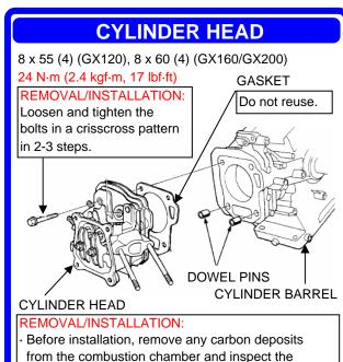
Measure the cylinder compression after reassembly.
