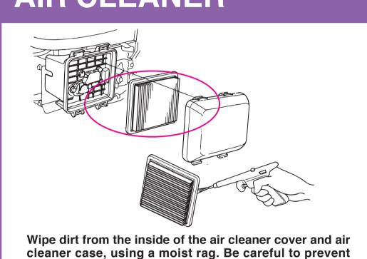
dirt from entering the air duct that leads to the
