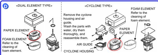
Paper element: Tap the element lightly several times on a hard surface to remove dirt, or blow compressed air (not exceeding 207 kPa, 2.1 kgf/cm², 30 psi) through the element from the inside. Never try to brush off dirt; brushing will force dirt into the paper fibers.
