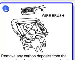
combustion chamber using a wire brush.
