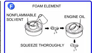
Excess oil will restrict air flow through the foam element and may transfer to the paper element, soaking and clogging it.
