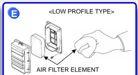
Wash the element in a solution of household detergent and warm water, then rinse thoroughly, or wash in nonflammable or high flash point solvent.
