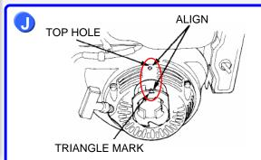
Set the piston at top dead center of the compression stroke (both valves fully closed).
