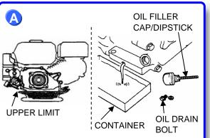
Insert the dipstick in the oil filter neck, but do not screw it in. Remove the dipstick and check the oil level.
