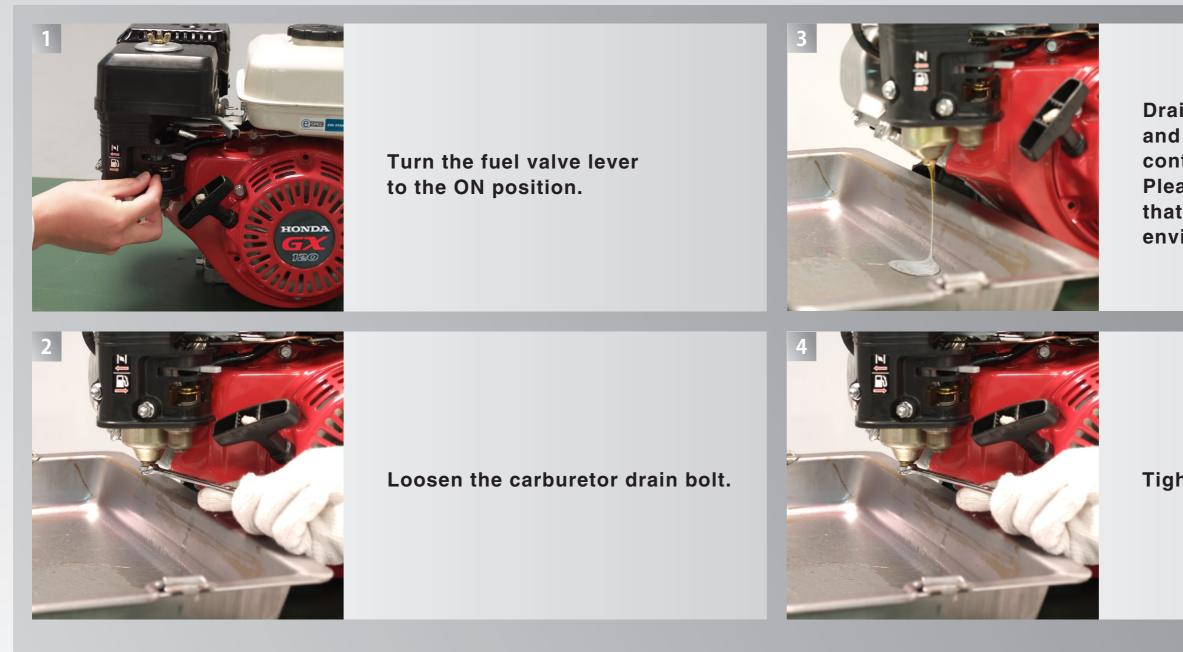
Drain the fuel from the carburetor and fuel tank into an approved container. Please dispose of fuel in a manner
